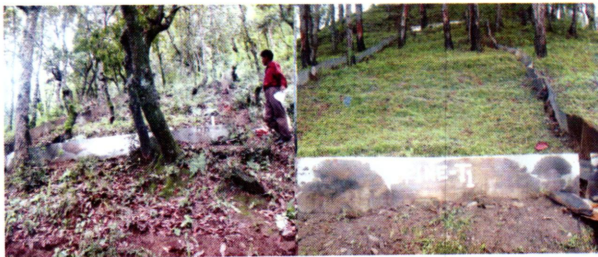
Fig. 39. Runoff plots maintained for hydrological studies under Oak (left) and Pine (right) forests
