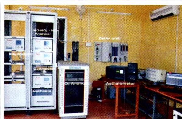
Fig. 46. Environmental observatory for monitoring gaseous and other aerosols at Mohal in the Kullu valley.
