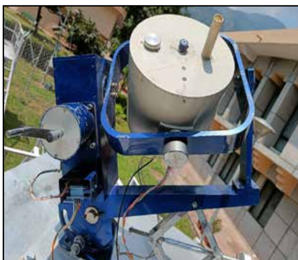
Fig. 20 Multi-wavelength radiometer (MWR) and sunphotometer set up for aerosol measurements at Mohal, HP
